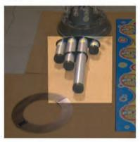
Step one: Remove the Waste Bin and Tube Holder from the machine.
