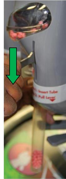
17. To remove the dispenser(s) first raise the top by rotating the header clockwise.
